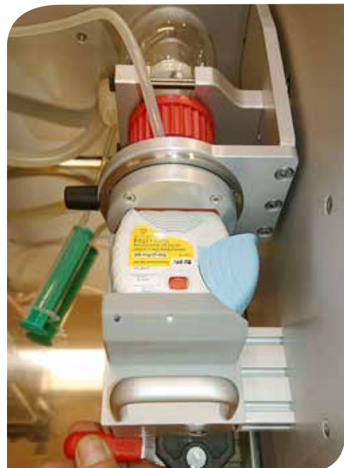
Figure 3. Customized Device Holders Purpose-built brackets hold inhalers tightly to the inlet of the glass frit impinger.
