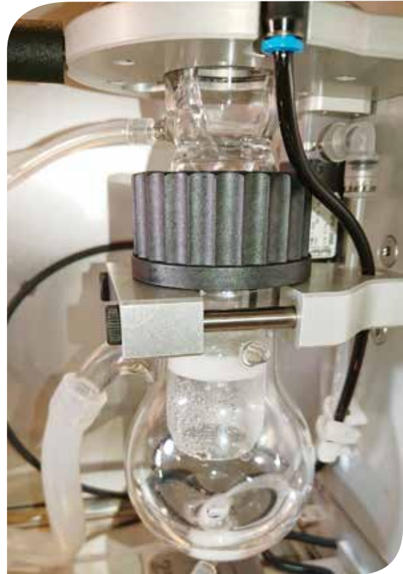
Figure 4. Pressure Tap at Inlet to Impinger
