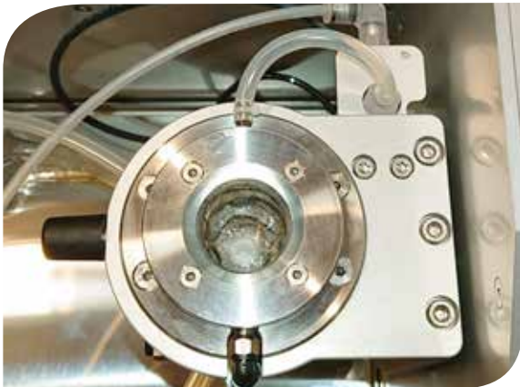
Figure 4. Pressure Tap at Inlet to Impinger
