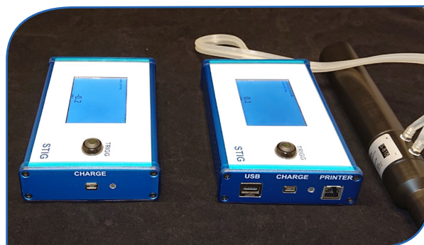
Figure 2. STIG consisting of control module and laminar flow element.
