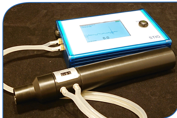
Figure 2. STIG consisting of control module and laminar flow element.
